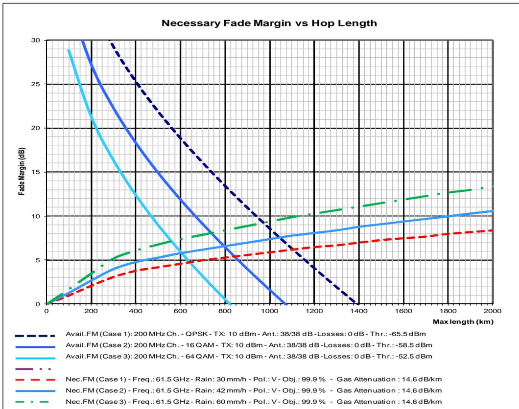
Figure 6.1.1.2: Maximum hop length, avail 99,9 %, 38 dBi antenna, QPSK to 64QAM
