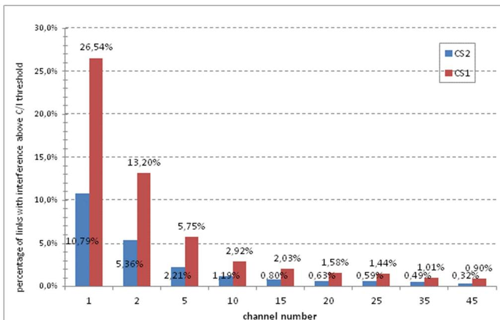
Figure 7.2.2.4: 32 dBi ETSI CS1 and CS2 classes comparison - 64QAM - DFS off
