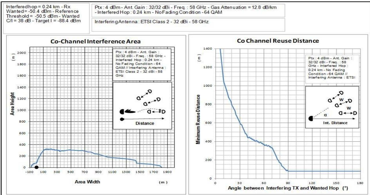
Figure 6.1.2.1: Protection area and distance for antenna 32 dBi and link length 240 m
