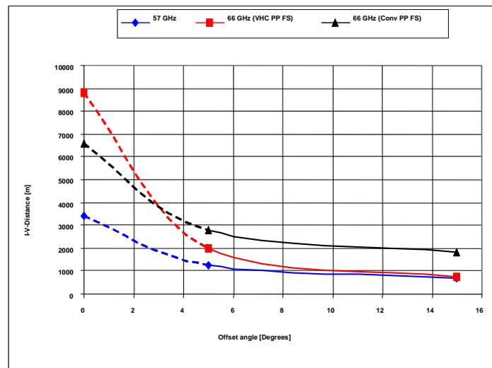
Figure 6.1.2.4: separation distances for FLANE Tx main beam to PP FS Rx (ECC Report 114 [i.6])
