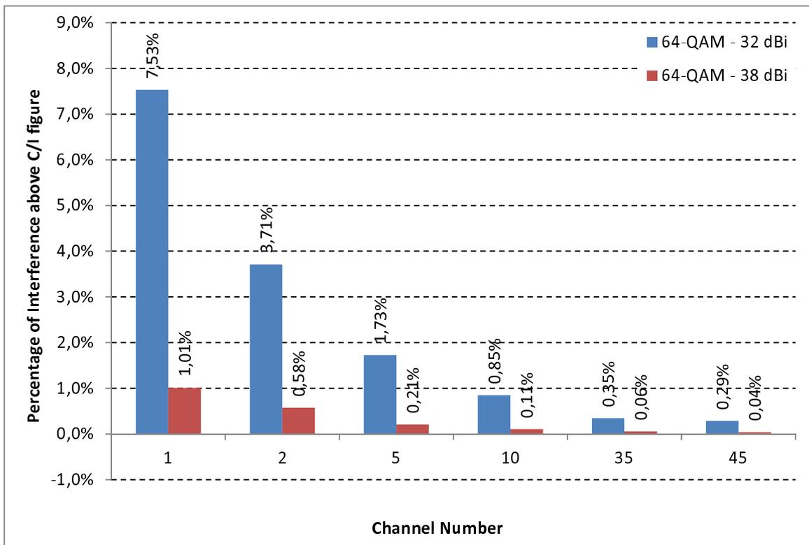
Figure 7.2.2.3: Summary of cases with FS systems only - ETSI based - 64QAM only- DFS on
