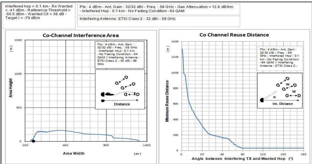
Figure 6.1.2.2: Protection area and distance for antenna 32 dBi and link length 100 m
