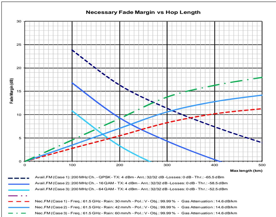
Figure 6.1.1.3: Maximum hop length, avail 99,99 %, 32 dBi antenna, QPSK to 64QAM
