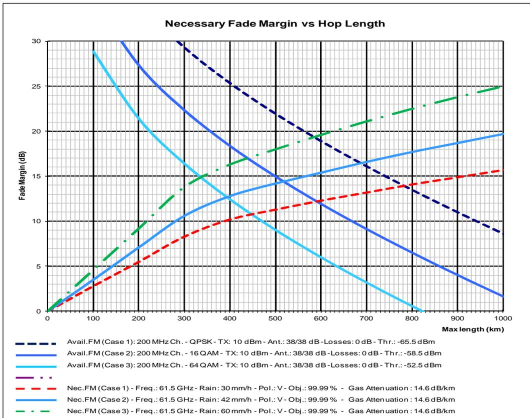
Figure 6.1.1.4: Maximum hop length, avail 99,99 %, 38 dBi antenna, QPSK to 64QAM
