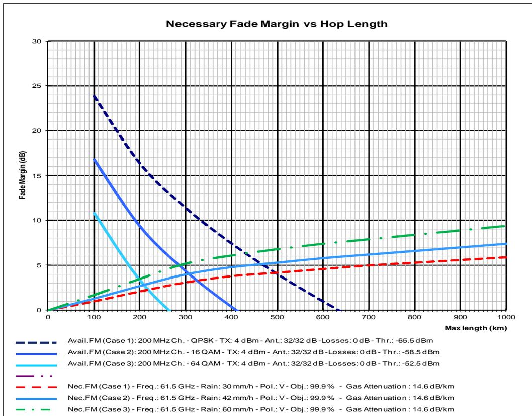
Figure 6.1.1.1: Maximum hop length, avail 99,9 %, 32 dBi antenna, QPSK to 64QAM
