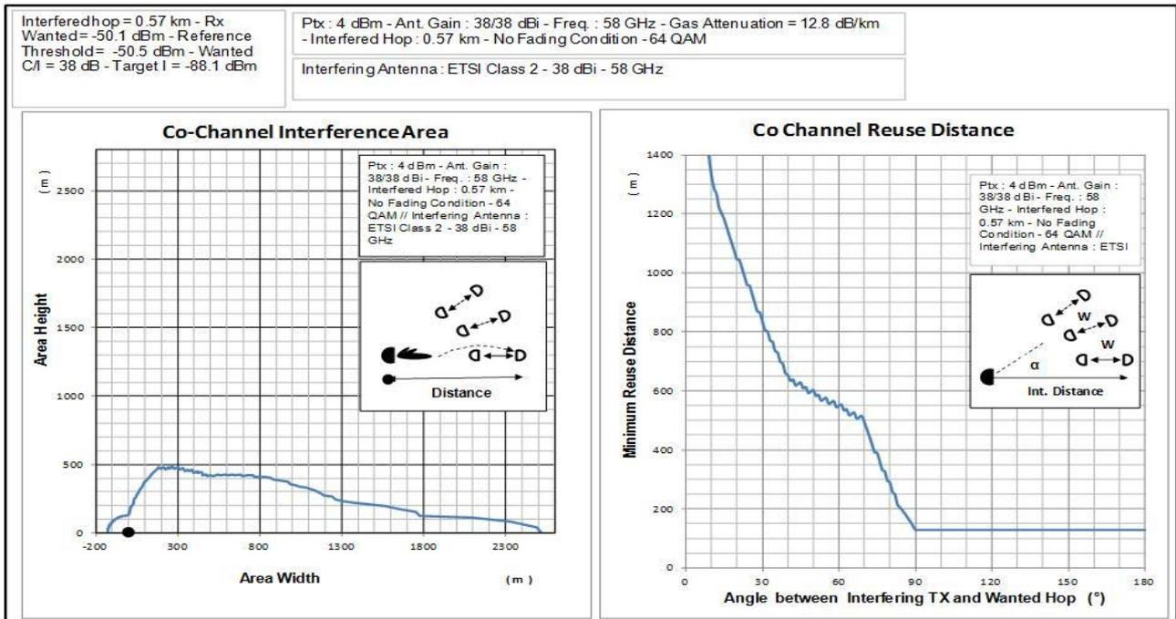
Figure 6.1.2.3: Protection area and distance for antenna 38 dBi and link length 0,57 km
